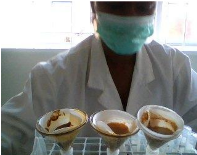
Figure 8. Lipid extraction using the Bligh and Dyer (1959) method
