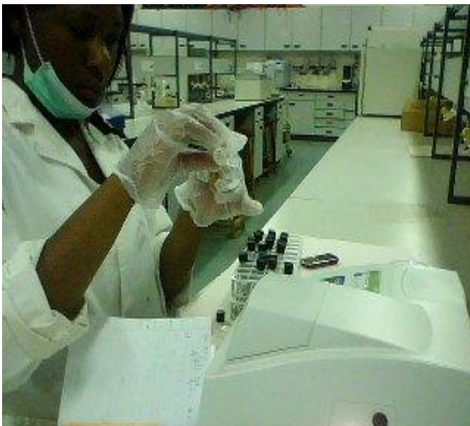
Figure 12. Student reading Absorbance values from a 'Genesys 20' Spectrophotometer
