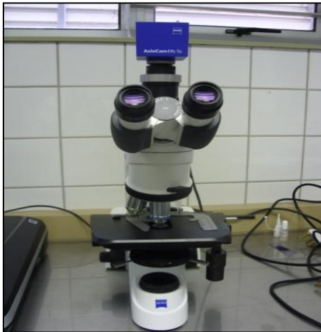
Figure 3: The 5 megapixel CMOS camera (AxioCameraERc. 5s) microscope – Photo: Lusia M. N. Negonga
