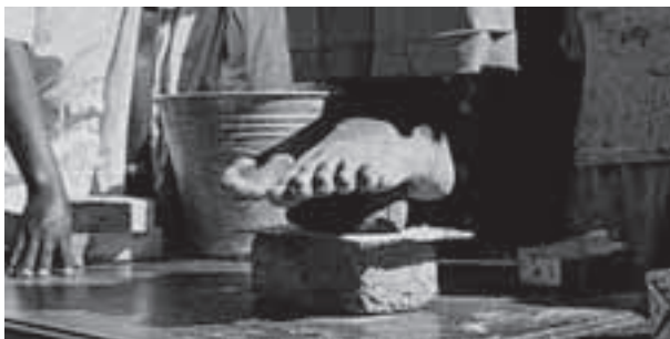
Determining the strength of a locally fired brick
