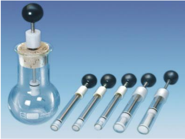
Figure 1.3. Plunger sampling pipette account to Hansen.
