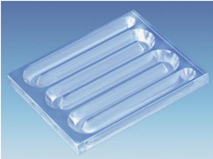
Figure.1.4. counting chamber for zooplankton; made of plexiglass with polished bottom for the best transparency and it has a dimensions 40 \times 70 (mm).
